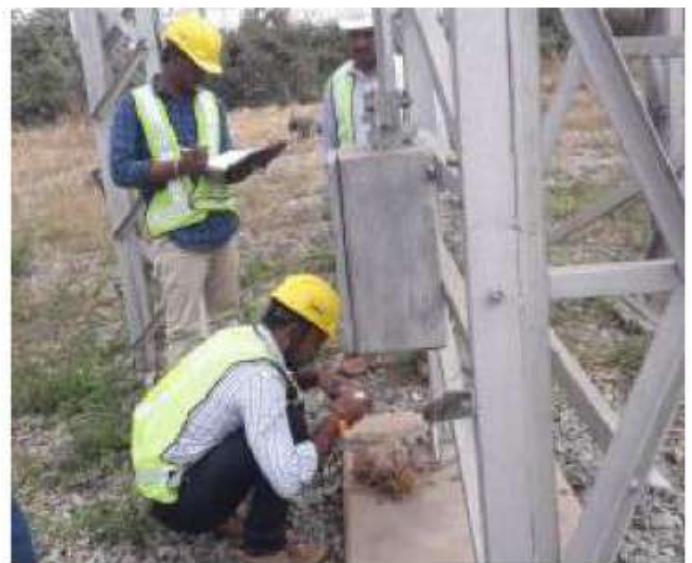
Rebound Hammer Testing (Civil input data collection) for structural design work - JUSNL Package 1 & Package 2 at Jharkhand.
